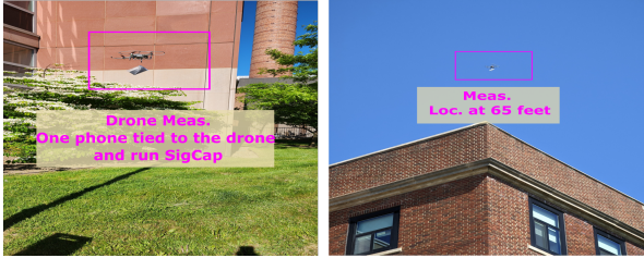
Figure 4: Drone measurement scenario.
