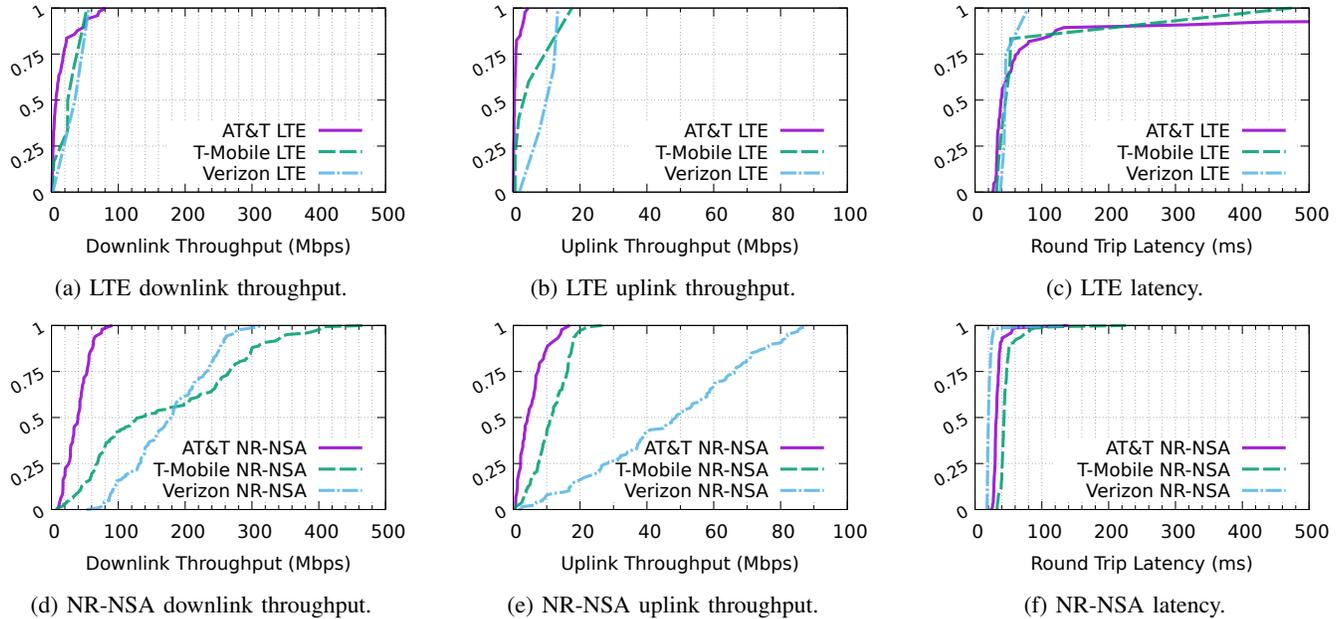
Fig. 8: Indoor survey of AT&T, T-Mobile, and Verizon in terms of throughput and latency performance.
