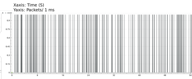
Figure 22: Disassociation Process on Fixed 20 MHz: LAA to Wi-Fi Coexistence
