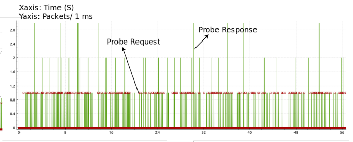
Figure 14: Probe Request and Probe Response on Fixed 20 MHz: LAA to Wi-Fi Coexistence
