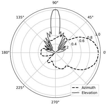
(a) Tx antenna directivity pattern  $G_{Tx}(\theta, \phi)$ .
