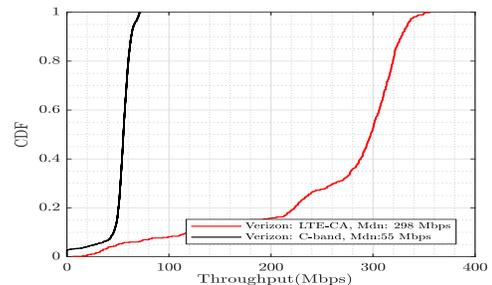
Fig. 15: Verizon LTE-CA and C-band throughput.
