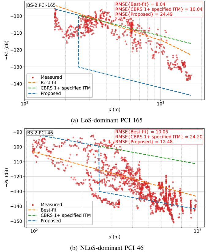
Fig. 17: Path loss analysis performed on LoS-dominant PCI 165 and NLoS-dominant PCI 46.
